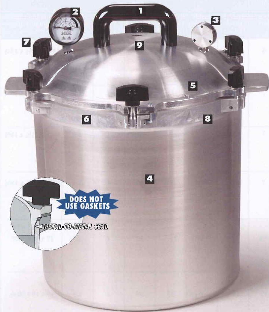
Only ALL-AMERICAN Pressure Canner/Cookers feature an exclusive, precision machined "metal-to-metal" sealing system. Positive action clamping locks align the cover to the base, forming a steam-tight seal. At the same time, this metal-to-metal seal automatically permits venting under unusual pressure conditions, providing an extra margin of safety over conventional rubber or composition gasketed cookers.
