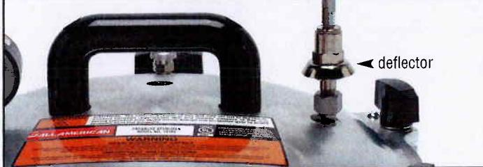
We have designed a new control valve that is larger in size and easier to operate. It now incorporates a protective deflector that directs and deflects any steam being released in a downward direction. By directing all of the steam downward whenever the unit is being exhausted, the operator is fully protected from the cloud of steam as it escapes.
