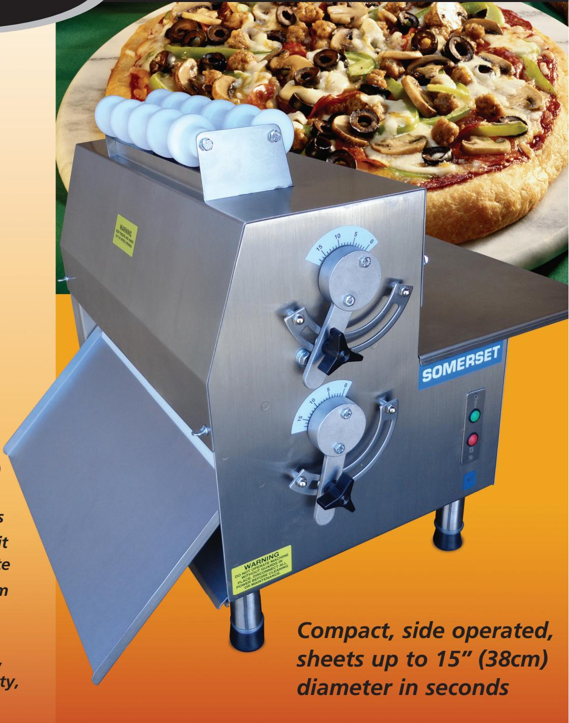
**Compact, side operated, sheets up to 15" (38cm) diameter in seconds**
